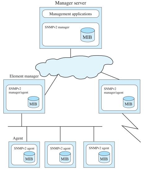
Figure 20.5 SNMPv2-Managed Configuration
